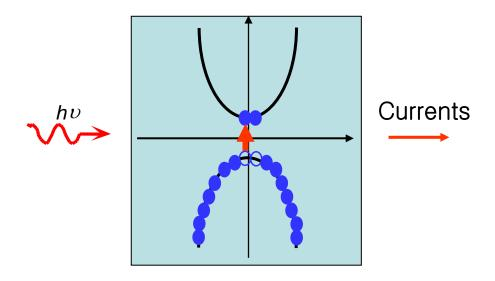
Materials for photodetection:  $E_g < h\nu$  Various methods for generating currents with photo-generated carriers: photoconductors, photodiodes, avalanche photodiodes
