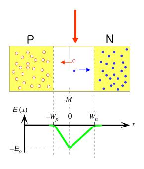
Photo-generated carriers drift into P (holes) and N (electrons) regions creating currents.
