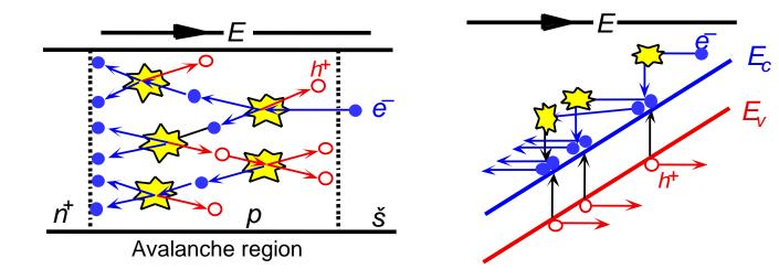
In real APD, care is taken so that only one type of carrier (either electron or hole) causes impact ionization.
